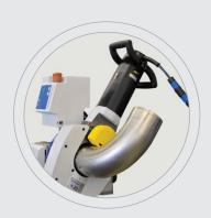
Ergonomically designed motor handle ideal for the cutting of elbows.
